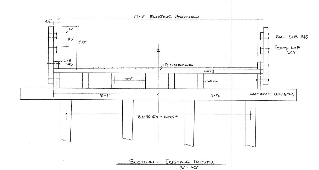
CRITERIA FOR H-15 LOADING - 6×16 STRINGERS C 2'-3" SPACING WITH 4" DECK - ADD 4 ADDITIONAL STRINGERS AS SHOWN FOR H20-5-16 LOADING
