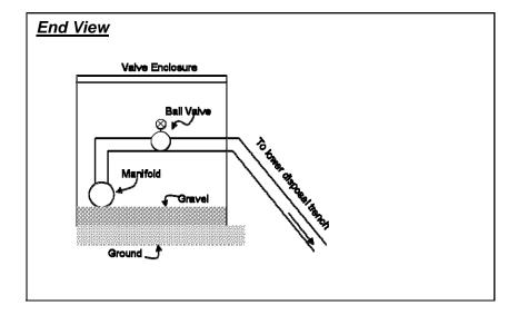
$\diamond$  The disposal trenches must be fed from the <u>top</u> of a manifold pipe.
