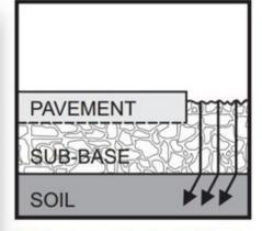
Potholes begin after snow or rain seeps into the soil below the road surface.
