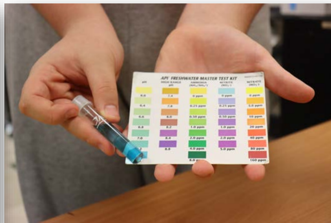
A student demonstrates how the water is tested regularly for pH, nitrates and ammonia as well as temperature.
